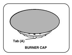
The Burner Cap top is porcelain enamel and has a tab (A) on the underside that fits into the notch (B) on the burner base (C).
